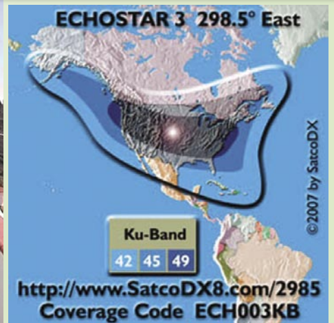
■ The footprint is far from reaching Europe – or so the theory goes. In the real world, reception is very well possible in the western fringes of Europe.
